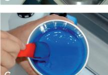
Weigh out an equal quantity of base and catalyst (e.g. 100 g of catalyst and 100 g of base; the end result is not affected by errors of up to 5%) mix vigorously until the product assumes a uniform color. Once the product is thoroughly mixed, pour it, preferably from 30 cm above the container, on to the one spot (this makes it easier for air to escape from the mix).
