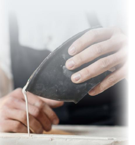
Zhermack condensation silicone allow to create a flexible silicone rubber mold (tin catalyst) that can be used to reproduce the object accurately and repeatedly.
