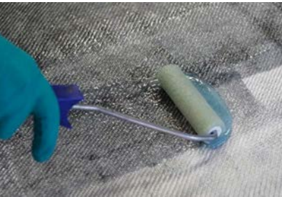
Wet lay-up with SikaBiresin CR168
