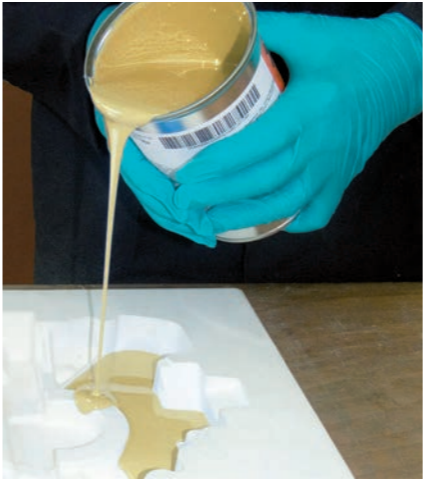
SikaBiresin® F160 with additional fillers for casting of models with thicker sections
