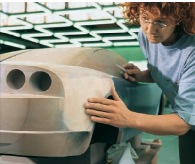
Models milled out of SikaBlock® PROLAB 65 N fulfil highest demands of surface quality
