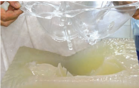
Demoulding of an optical part made of SikaBiresin® PX521 / PX522
