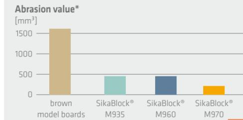
\* Standardised abrasion test for elastomeric resins [ISO 4649] - the lower the measured value (abrasion in mm³) the higher the abrasion resistance.
