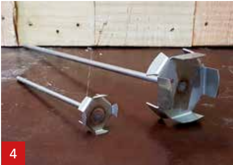
4 Use the A1 mixer. Small: up to 1.5 kg of A1. Large: 1.5 kg or more A1.
