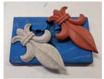
Result after drying and unloading; a solid cast object, an exact copy of the mould.
