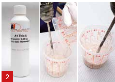
2 Add 2% Thix A (of the total quantity A1) to the A1 Liquid. By using Thix A the A1 will result in a thicker texture.
