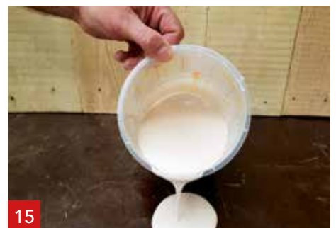
15 A1 is ready for laminating, casting or spraying. Processing time 20 - 25 minutes.
