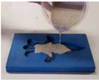
Pour part of the created A1 into the mould. Start (if possible) by brushing the mould, so all unevenness/relief is touched with A1.
