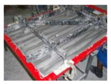
A frame is used to position the mounting brackets on the finished laminate.
