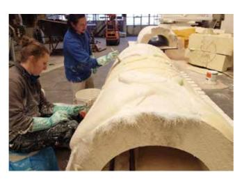
Impressive concrete elements are designed which require an impressive support construction. The alternative is blocks of EPS covered with several layers of glass fibre reinforced A1. By adding pigments and sand to the A1 a concrete feel and look is achieved resulting in a lightweight By: Decolite impressive 'concrete' façade.
