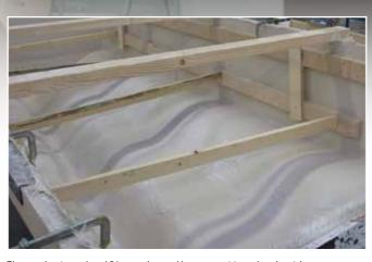
Element laminated and 36 mm plywood beams positioned to the sides
