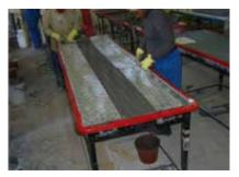
Apply the 1st laminate layer: A1 with 2 layers of A1 Triaxial fibre.
