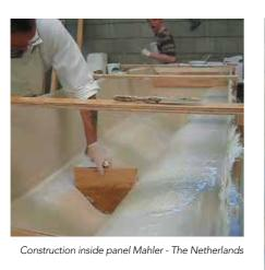
To attach reinforcement materials, gluing can be done by laminating with A1 and Triaxial fibre. It is also possible to glue materials with bonding products. Observe the manufacturer's instructions. Excellent adhesives include MS polymer sealants.
