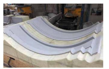
From the scanned data, a 3D-model has been made with all 35 A1-elements to be made. For each element to be made a direct mould has been produced by Nedcam. The direct moulds were made of an EPS-base with a PU-paste layer that was milled to the exact dimensions.
