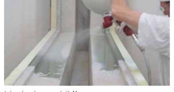
L-shaped panels are sprayed with A1.
