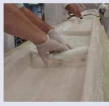
To laminate, you have to work wet in wet. A quick way to apply A1 is with a brush or roller.
