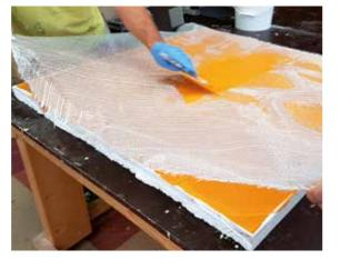
Before applying the A1 Triaxial fibre, cut it to size first, given the processing time of A1.
