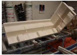
Within 2 hours the panel is demoulded for futher curring. On the inside panels are being reinforced with aluminum.
