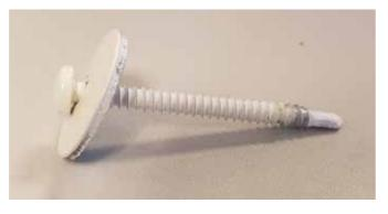
In the project the maximum distance of the screws is selected to be 500 mm. Moreover, the maximum distance of screws near the end of the profile is selected to be 90 mm. Because the lengths of the elements vary, sometimes the distance between two screws is less than 500 mm. A typical screw pattern in the project is illustrated. These ventilation openings are realized by placing 3 mm EPDM-rubber strips between the element and the building during mounting. **cross-section detail**
