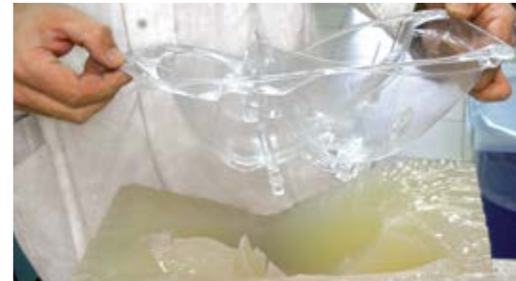
Elastic mould made of addition curing silicone Essil 291 for optical parts
