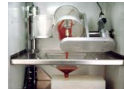
Vacuum casting process provides parts with best visual appearance and highest mechanical properties
