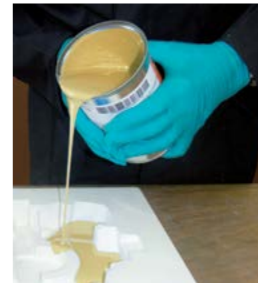
F160-1 with additional fillers for casting of models with thicker sections
