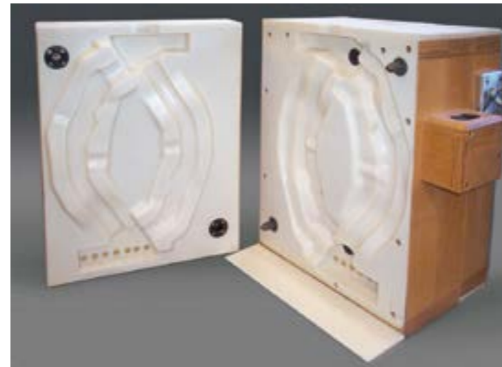
Core box made of Biresin® U1320 NT
