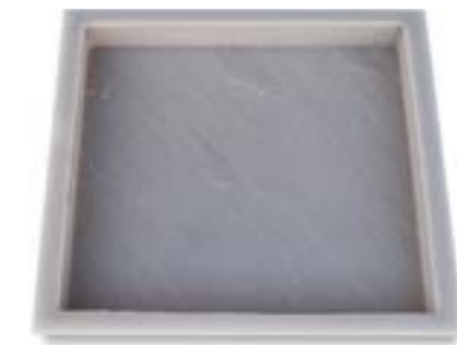
Mould out of UR58630 for concrete casting
