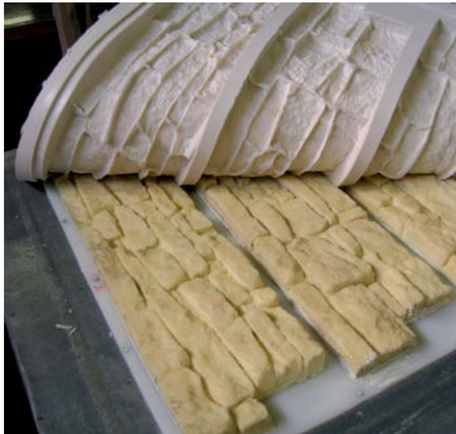
Release of UR 58480 soft mould for stone facing
