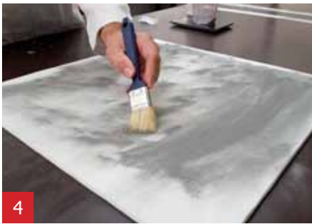
Rub the iron powder with a (dry) brush in to the mould.
