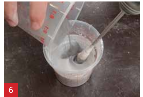
Then add the remaining iron powder to the A1 and stir for 1 minute.
