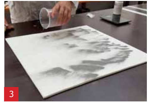
Spread 25 g of the iron powder over the mould.
