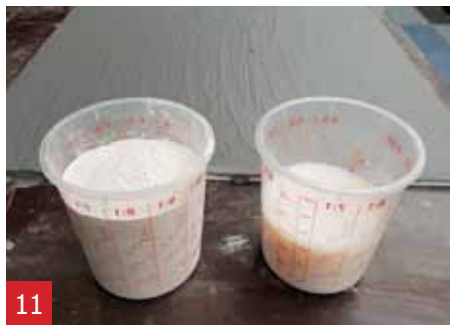
When the panel is dry, weigh 900 g A1 powder and 450 g A1 liquid.
