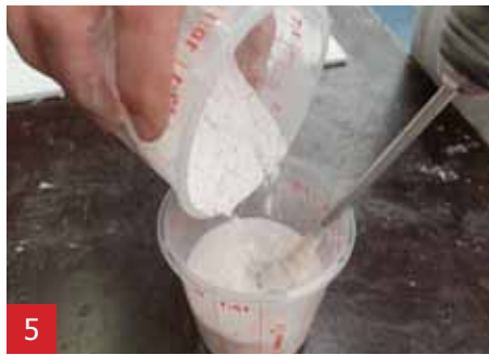
Add the A1 powder slowly to the A1 liquid and stir with the mixer until you have a smooth surface.
