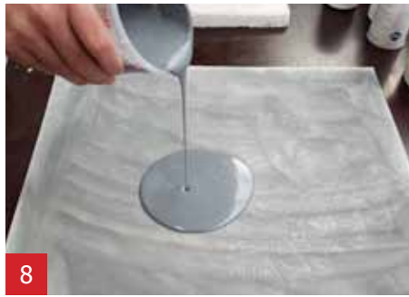
Apply the A1 onto the mould and spread with a brush.
