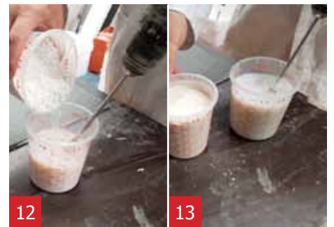
Again add the powder to the liquid and mix for 1 minute 12 . Directly clean the mixer in water 13 .
