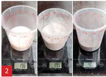
Calibrate the scale and weigh 200 g liquid, 400 g powder and 400 g iron powder.
