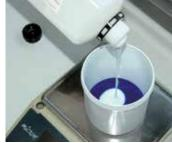
Weigh out an equal quantity of base and catalyst (e.g. 100 g of catalyst and 100 g of base; the end result is not affected by errors of up to 5%)
