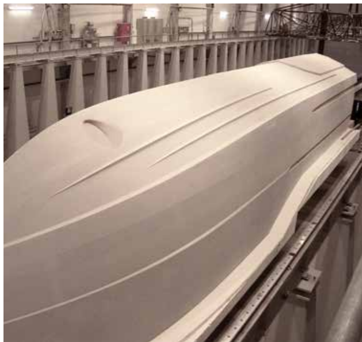
43 m long boat hull made of SC175 with a perfectly smooth and seamless surface
