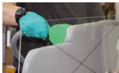
SC175 thixotropy enables vertical application in single layer and without sagging
