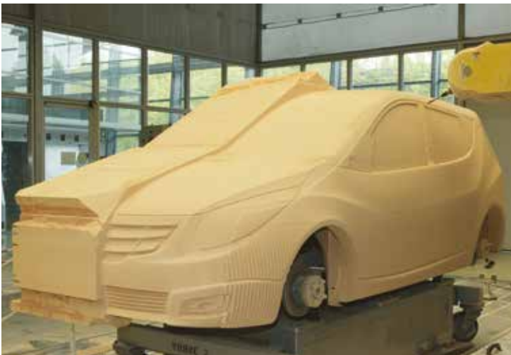
Full scale car model made of SikaBlock® M330 boards bonded with Biresin® Kleber Orange
