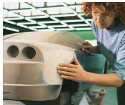
Models milled out of Prolab 65/70 fulfil highest demands of surface quality
