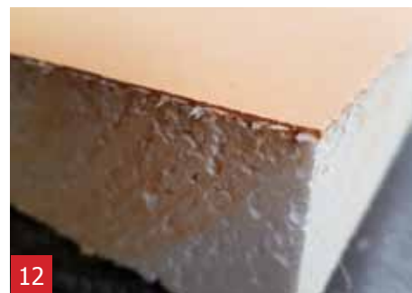
11 Final result, a strong panel coated with a thin layer of A1.
