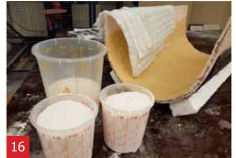
In the meantime weigh 450 g liquid and 900 g powder. Also cut 4 pieces of triaxial fibre same size as the mould you will be using.
