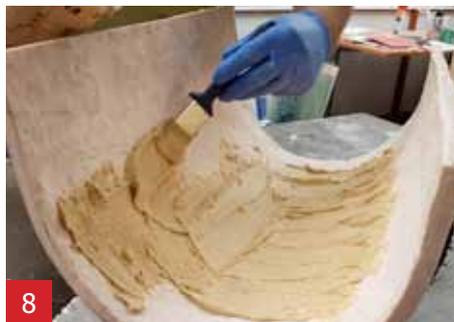
8 By using Thix A the A1 becomes thicker, like a gelcoat and the A1 won't drop down from the vertical parts.
