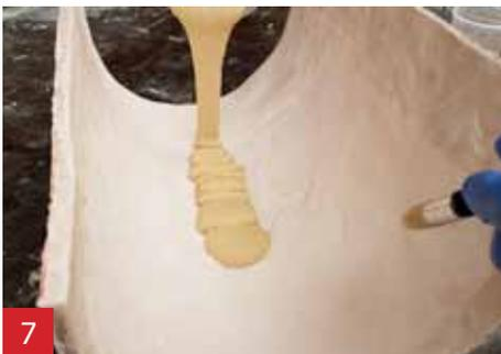
7 Apply the A1 with a brush in the mould.
