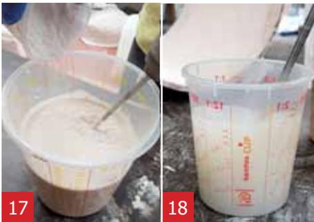
Add the A1 powder slowly to the A1 liquid and stir with the mixer until you have a smooth mixture **17**. Clean the mixer directly after use in water **18**.
