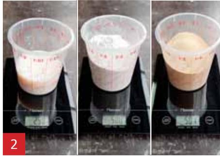
2 Calibrate the scale and weigh 250 g liquid, 500 g powder and 500 g yellow sand.
