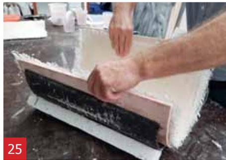
Take the silicone mould carefully from the support mould.
