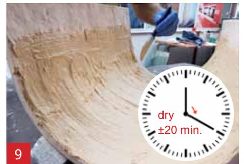
9 The surface must reach a thickness of 3 mm. Let the panel dry for  $\pm 20 \text{ min.}$
