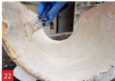
Again apply a thin layer of A1 and smoothen the A1 over the surface.
