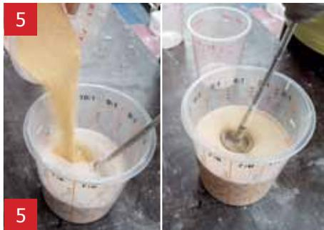
5 Add sand to the A1 and stir well. Also add 5 g Thix A to the mixture of A1 and sand.  $(250 \text{ g} + 500 \text{ g} = 750 \text{ g} + 0,5\% = 5 \text{ g})$
