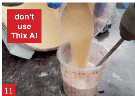
11 For the 2nd layer of A1 we weigh 125 g liquid, 250 g powder and 250 g yellow sand, and mix them as in step 4 and step 5.
