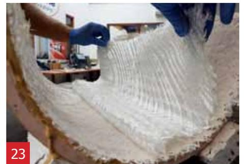
Apply another layer of triaxial fibre. Repeat step **21** and **22** until you have 4 layers of triaxial fibre. When finished clean the brush with water.
