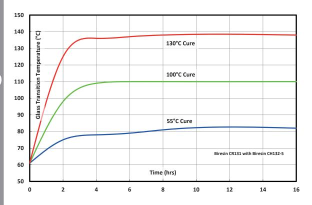
When curing a composite part, the whole of the part (including the very middle of the laminate) needs to see the cure temperature.
