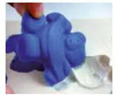
Mix vigorously until the product assumes a uniform colour. Once the product is thoroughly mixed, pour it, preferably from 30 cm above the container, on to the one spot (this makes it easier for air to escape from the mix). **These instructions apply only to RTV2 poly addition silicone rubbers.**
