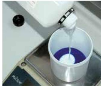
Weigh out an equal quantity of base and catalyst (e.g. 100 g of catalyst and 100 g of base; the end result is not affected by errors of up to 5%)
